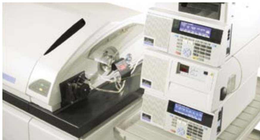
Speciation analysis is accomplished with the PerkinElmer Series 200 HPLC system performing the separation and the PerkinElmer SCIEX ELAN providing detection.
